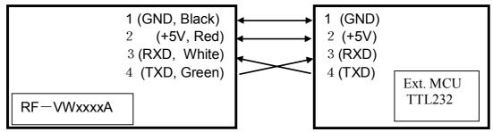
Note: VWxxxxA -232T's interface voltage level is TTL. When connect to a PC, a external voltage converter, for example, Max232 can be used.
